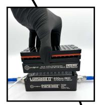
Seal the inserts with the reactor block lid and place on top on the illuminator for bottom-side illumination.
