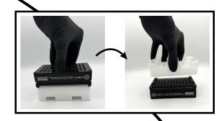
Load OWiC SPECS for 1 ML inserts into the reactor block either manually or by flipping all 96 into the reactor as shown.
